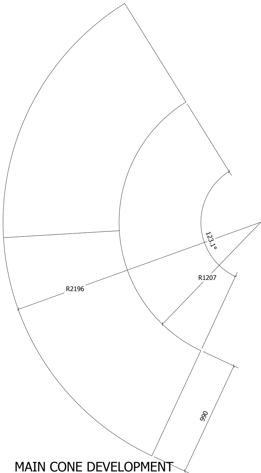
MAIN CONE DEVELOPMENT 3mm MILD STEEL
